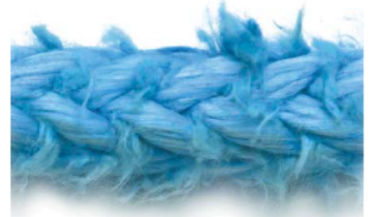
Severely abraded rope.
